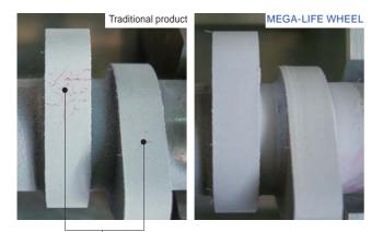
Areas with grinding cracks Fig. 4 Grinding test results (cracking inspection)
