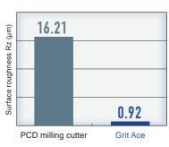
Fig. 4 Surface roughness
