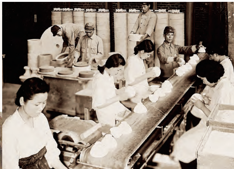
Firing plant for mixed-firing of tableware and grinding wheels (around 1940)
