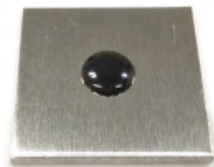
New glass material successfully prototyped (heated at 300°C and joined with aluminum)
