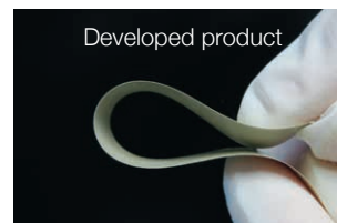
Conductive resinous silver paste after heat-resistance testing (200°C for 10 hours)
