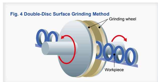
Recently, market demand has increased for simultaneous grinding using multi-axis grinding machines.
