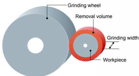
$$Q'(\text{mm}^3/\text{mm}\cdot\text{s}) = \frac{\text{Volume of workpiece removed}(\text{mm}^3)}{\text{Grinding width}(\text{mm}) \times \text{Cycle time}(\text{s})} \dots\dots\text{Equation 1}$$
