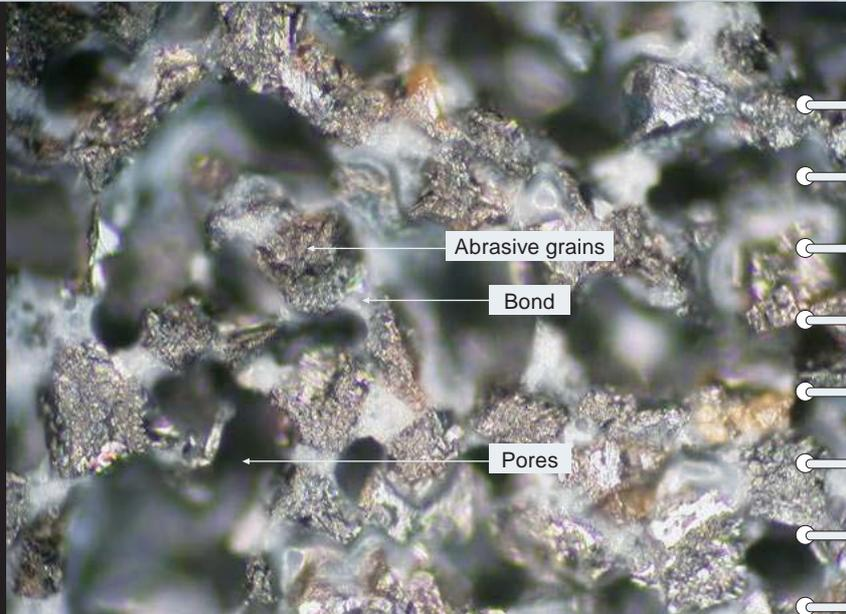
Fig. 1 Grinding wheel photo (vitrified-bond CBN wheel)
