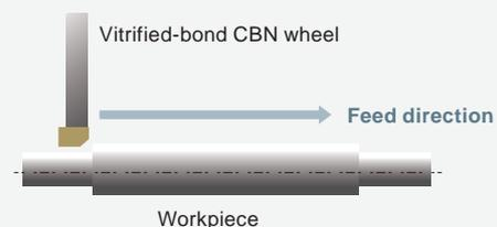
**Fig. 10 Contour grinding test method**
