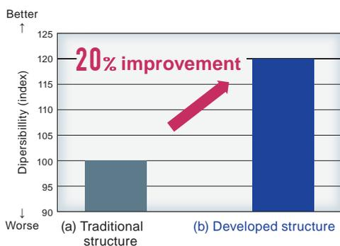
**Fig. 8 The dispersibility of CBN gains in grinding wheels**
