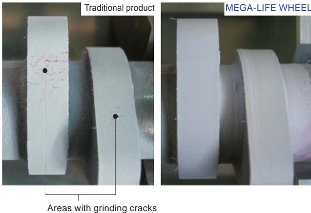
Fig. 4 Grinding test results (cracking inspection)
