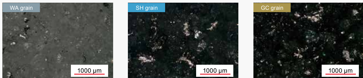
Fig. 6 Grinding Wheel Surface Condition after Grinding
