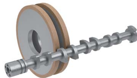
Fig. 1 Outline of Cam lobe grinding
