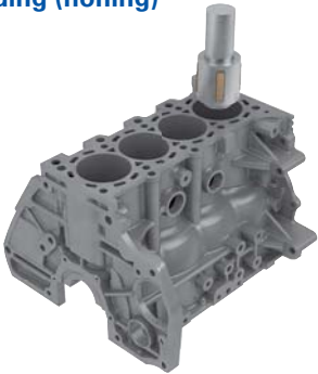
Fig. 6 Schematic diagram of cylinder bore grinding (honing)
