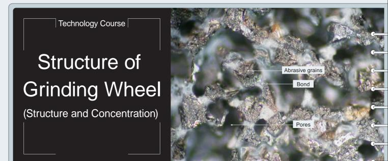
Fig. 1 Grinding wheel photo (vitrified-bond CBN wheel)
